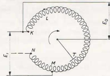
Fig. 7—Diagram of variable transformer showing normal connection.
