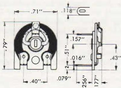
Fig. 5—Type E097AA/. Both track and contact terminals are soldering lugs for direct soldering into the wiring. The potentiometer can be fixed using the hole provided.
