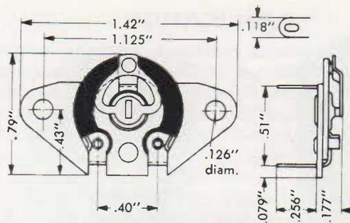
Fig. 6—Type E097AE/. Both track and contact terminals are soldering lugs for direct soldering into the wiring. The provision of two mounting holes makes this type particularly suitable for screw mounting to the back of a TV or amplifier chassis.
