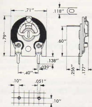
Fig. 2—Type E097AB/. Track terminals are pin connections for mounting the potentiometer perpendicularly to a printed board; contact terminal is a soldering lug.
