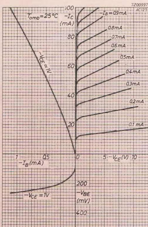
Fig. 5—Typical characteristics of AC 125.
