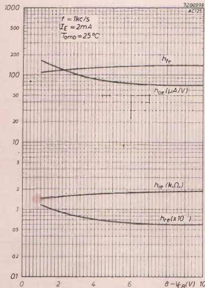
Fig. 8—Typical variation of h-parameters with collector-base voltage for AC 125.
