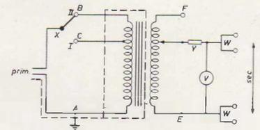
Fig. 9—Circuit diagram of bench-mounting types (Y is protective fuse).
