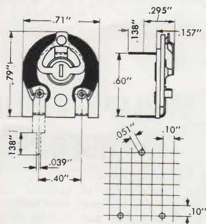
Fig. 4—Type E097AD/. Both track and contact terminals are pin connections for mounting the potentiometer parallel to a printed board.
