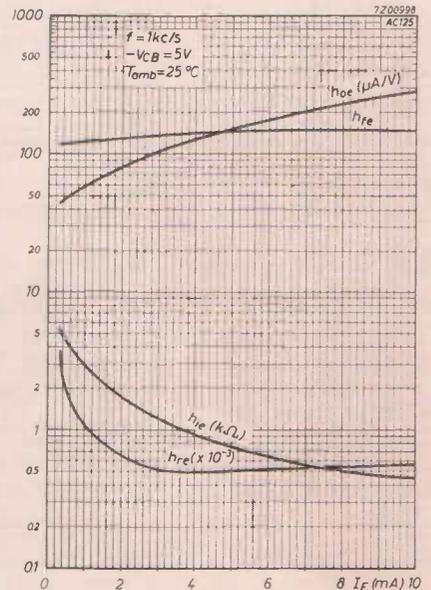
Fig. 9—Typical variation of h-parameters with emitter current for AC 125.
