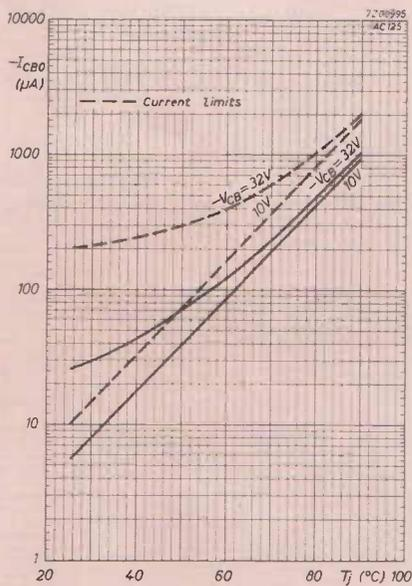
Fig. 7—Collector-base cutoff current of AC 125 and AC 126 (max. and typical values).
