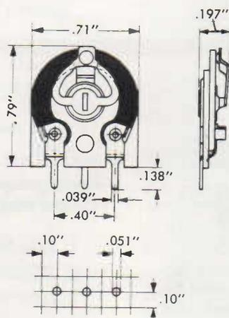
Fig. 3—Type E097AC/. Both track and contact terminals are pin connections for mounting the potentiometer perpendicularly to a printed board.
